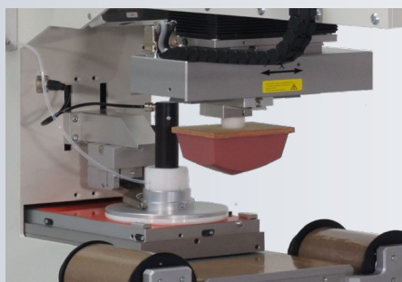
optional pad movement for lateral tampon movement
