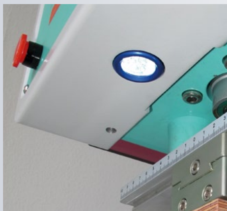
LED light for work area
