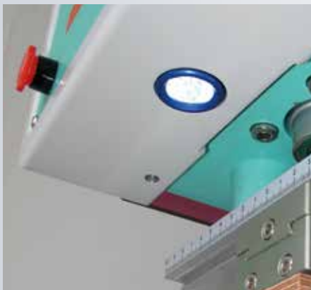
LED light for work area
